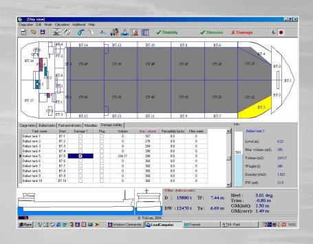
Typically these conditions are identified by the compartment(s) damaged ex: "Water Ballast Tank 5 Stb"
