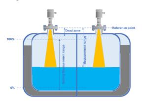
Measuring reference is the sealing surface of a flange.
